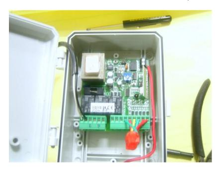
STEP 3: INSTALL AN ANTENNA 16CM LONG ON TERMINAL NUMBER 15.
