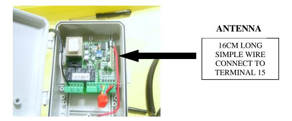
STEP4: TO INSTALL MOTOR CONNECT MOTOR WIRES TO TERMINAL 4, 5, 6.
